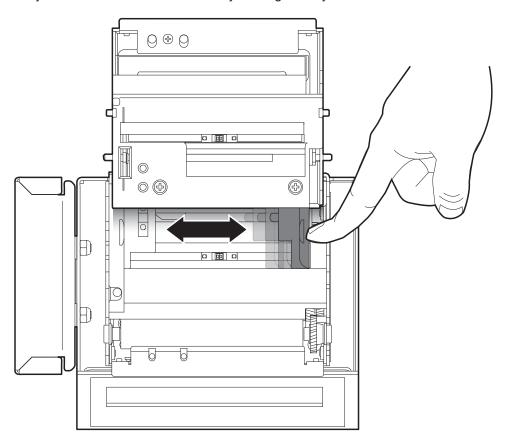
To manage paper width from 20 mm to 25 mm, apply the spacer on the mobile paper guide (see following figure), then adjust the paper width.
