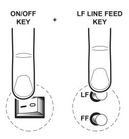
While pressing the LF LINE FEED key, switch on the device by pressing the ON/OFF key.
