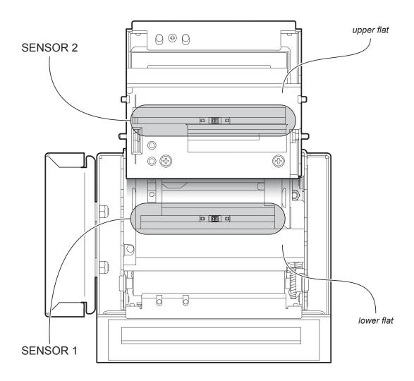
The following figures show the usable format of paper and the corresponding sensors used for alignment:
