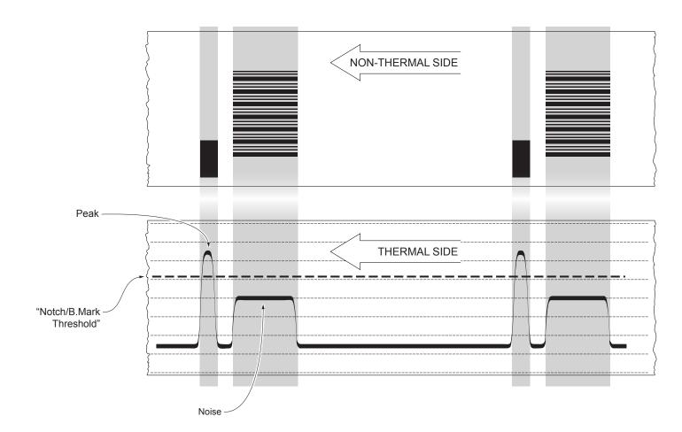
If the maximum value of "noise" read by the sensor is very close to the peak value, it might be difficult to place the value of the "Notch/B.Mark Threshold" at an intermediate point. In these cases, it is mandatory that the portion of paper between the point of printing end and the front notch is completely white (no graphics). In this way, the only next graphic detected by the sensor for alignment after the printing end will be the notch.
