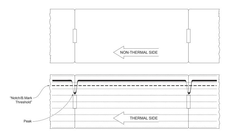
The following figure shows an example of paper with the non-thermal paper printed with black marks and other graphics (for example, a barcode): the outgoing voltage is constant while passing the white paper between two notches, presents a peak at each black mark and presents some "noise" at each barcode. In this case, the optimal value for the "Notch/B.Mark Threshold" parameter is located about halfway between the peak value and the maximum value of the "noise".
